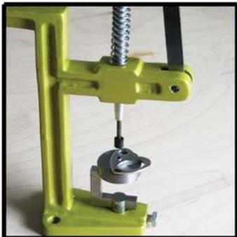
The Unilock Press can be screwed half-way out from the edge of the bench in order to accommodate bangles and other large rounded forms that can rest with their top part over the jig base and the lower part hanging under the press. Jig base supports are needed for this operation.
